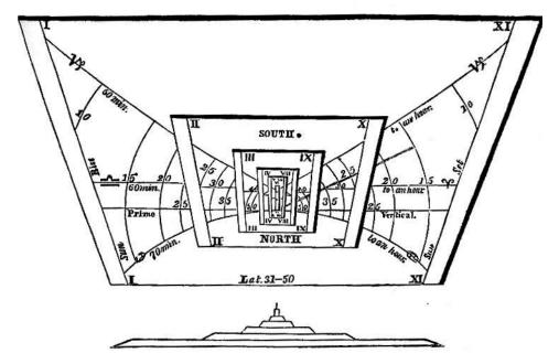
7. A description of the dial. This dial consists of eleven steps placed parallel to the horizon, with a perpendicular gnomon fixed in the upper or middle step, which step is placed exactly north and south, and forms the meridian or sixth-hour line.
